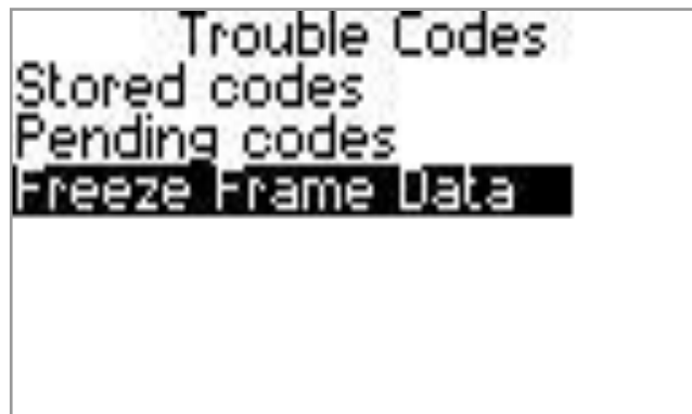
Fig. 2.6.1: Engine operation parameter values recorded at the moment when a fault has occurred.
