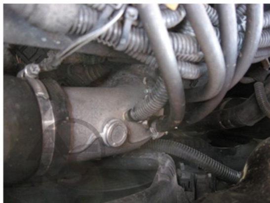
Photo 8 Positioning of the common nozzles after the turbine
