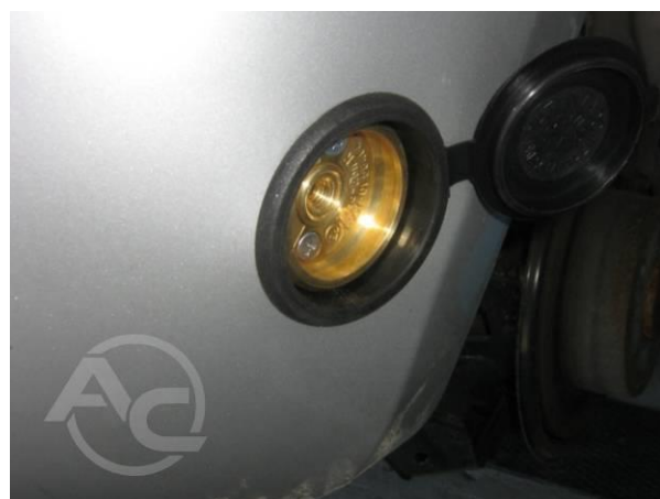
Photo 2 . Installation of the LPG filling valve
