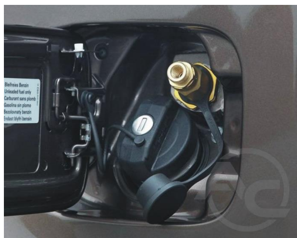
Photo 2 . Installation of the LPG filling valve
