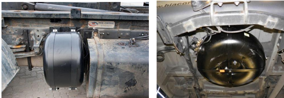
Photo 4. Installation of the LPG tank
