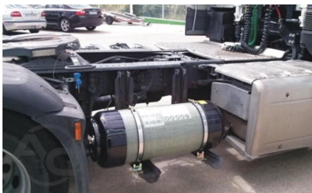
Photo 4. Installation of the LPG tank
